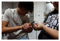
working. If the wiring was to be cut too short, our robot would circuit. The wiring is very essential to the robot which is why we had to be very cautious with how much we were cutting off and how we were wiring. After finally stripping all the wires our electrical members were making sure to tightly seal up the wires so they were waterproof.
